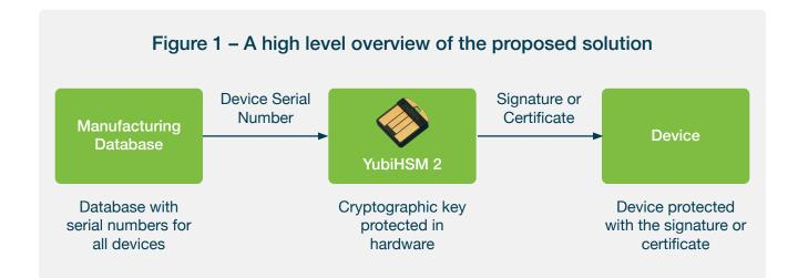
*Figure 1* (above) provides a high level process summary of the proposed solution to be implemented, as either a replacement or a brand new process in manufacturing plants and/ or production lines, with the YubiHSM 2 at the core. The foremost point to highlight is that the cryptographic key used to sign and/or certify components is never exposed *outside* of the YubiHSM 2 hardware, thus ensuring a high level of security.
