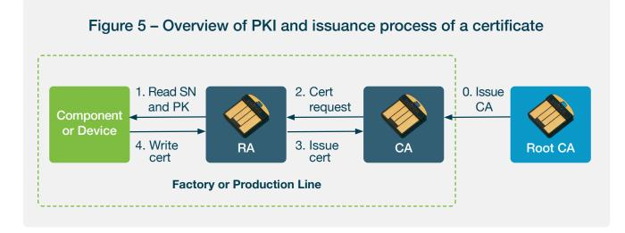
Under the illustrated design, the Root CA uses a YubiHSM 2 to house its key-pair (i.e. both its Private and Public Keys) in addition to its certificate. Due to the diminutive size of the YubiHSM 2, the Root CA server can practically be located anywhere, although traditionally, the Root CA is hosted in an offsite data centre for security reasons, but also due to the tremendous physical size of server farms and a typical HSM.
