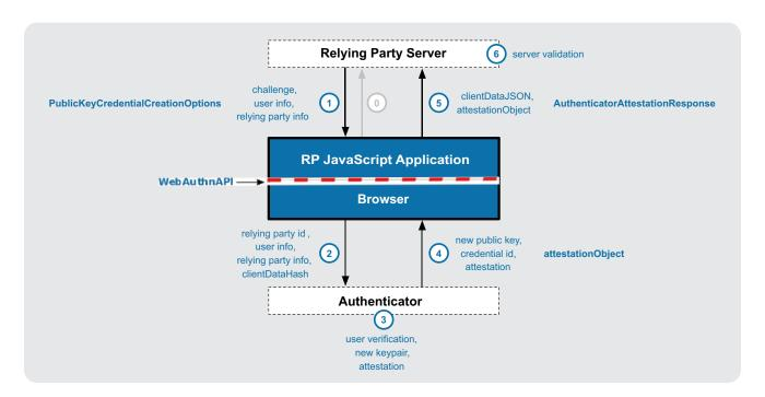
Including a domain in the challenge prevents other sites from spoofing the relying party. For example, if a phishing site were to send the user a challenge with demo.yub1co.com, the client/platform would recognize the discrepancy and authentication would fail.
